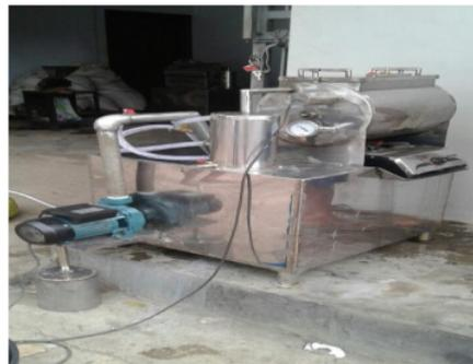
Gambar 1. Mesin Vacuum Frying Kapasitas 2 Kg Bahan
