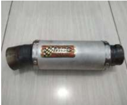
Gambar 4 Silencer Knalpot Model Oval
