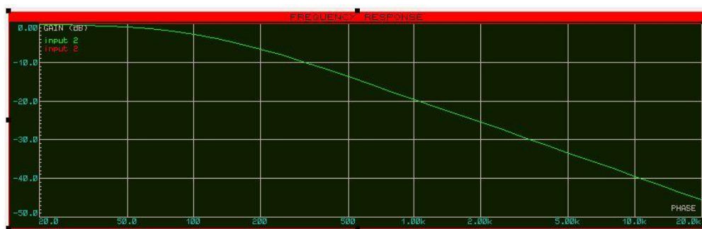
Gambar 4. 4 Respon Frekuensi Output Rangkaian Low Pass Filter
