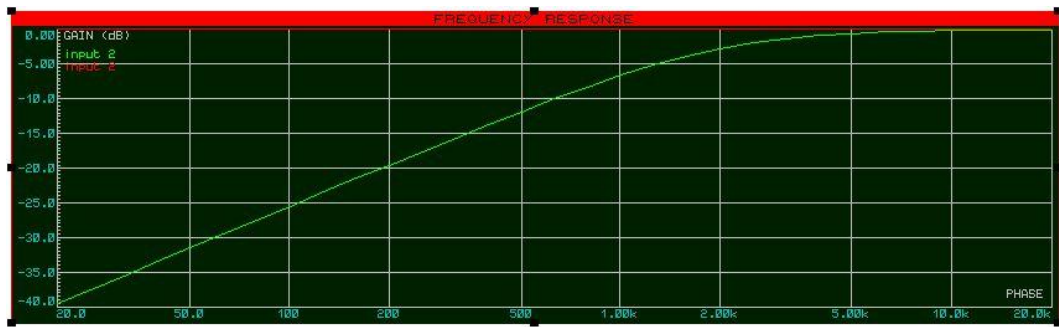
Gambar 4. 2 Respon Frekuensi Output Rangkaian High Pass Filter
