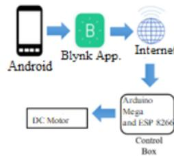
Figure 1. Overall System Diagram
