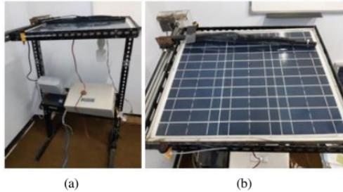
Figure 3. Wiper cleaner prototype (a) side view (b) top view
