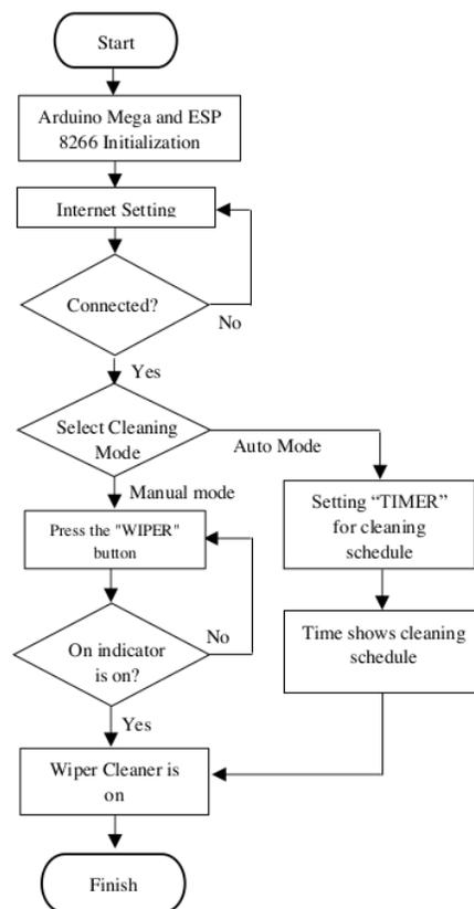
Figure 2. Flowchart of Wiper Cleaner System
