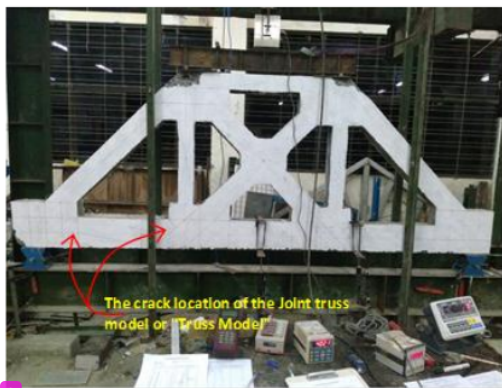
2 Fig. 7. The crack pattern of the joint truss model or "Truss Model"
