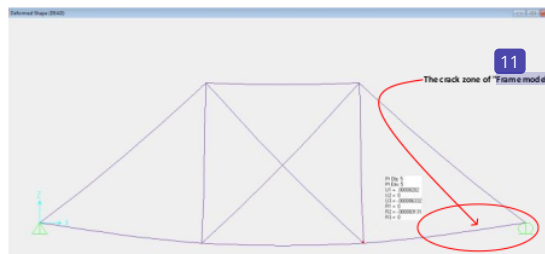
Fig. 10. The deformation of the rigid portal model or "Frame model"
