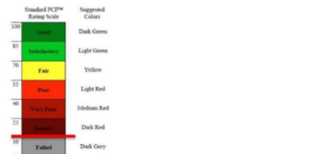
Gambar 3. Diagram Nilai Pavement Condition Index. (shahih, 1994)
