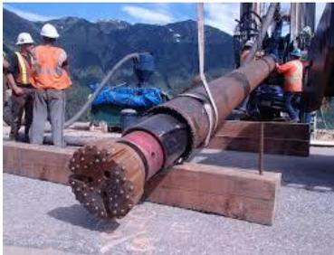
**Gambar 5.7. Down-Hole Hammer Drill**
