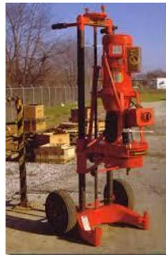
**Gambar 5.2. Bor mesin ringan (*portable drilling rig*)**
