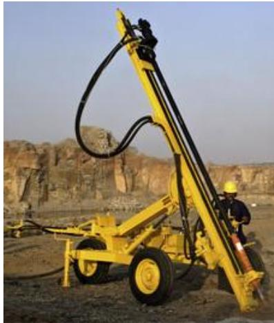
**Gambar 5.6. Bor Palu (*Hammer Drill*)**
