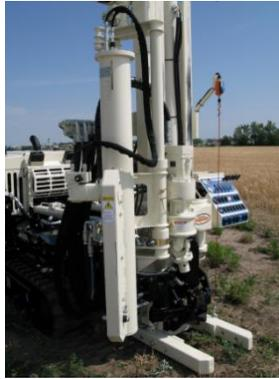
**Gambar 5.8. Hammer Drilling Rig with Drive Sampler**
