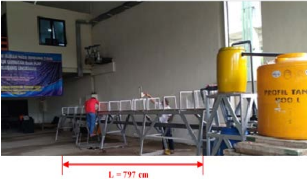
Fig.2 Physical model of open channel to get the discharge coefficient constant ( C_d )
