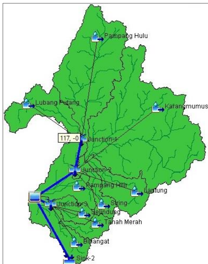
Figure 9. The modeling system of Hydrology in Karangmumus watershed using HEC-HMS
