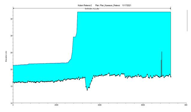
Fig. 9: Profile of the water level passing through the city of Barabai with a discharge of 60% of the Planned Discharge. (Source: Calculation Result, 2021)
