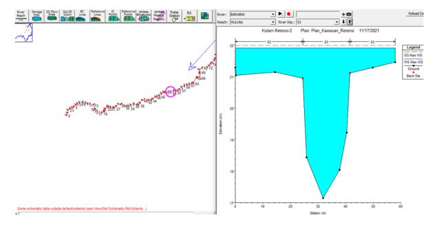
Fig. 11: Water level profile at STA 53 with 60% discharge. (Source: Calculation result, 2021).
