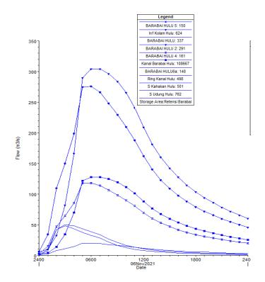
Fig. 5: Calibrated flood hydrograph. (Source: Calculation Result, 2021)
