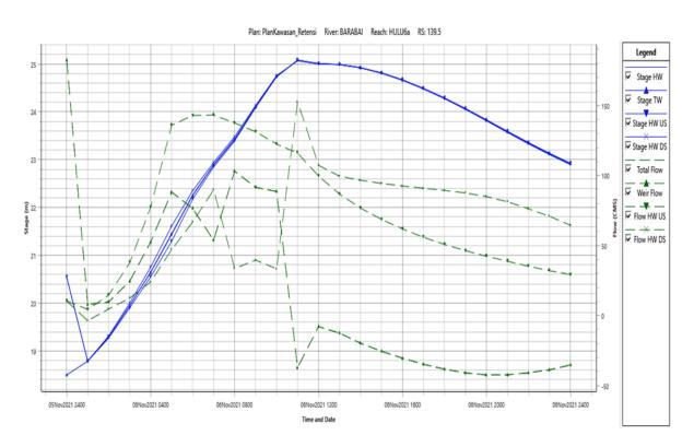
Fig. 8: Simulation of flow profile on side spillway with 40% discharge. (Source: Calculation Result, 2021)
