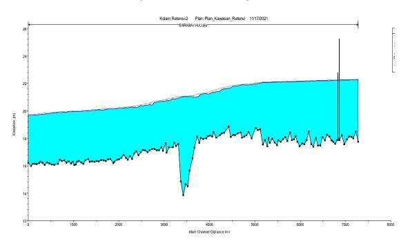
Fig. 14: Long section and cross conditions section after repair. (Source: Calculation result, 2021)
