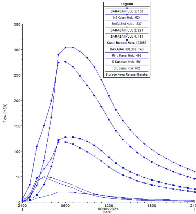
Fig. 5: Calibrated flood hydrograph. (Source: Calculation Result, 2021)
