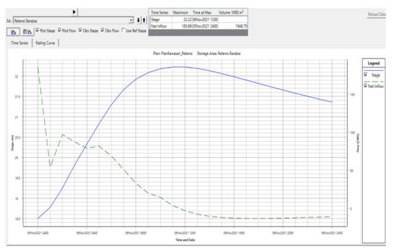
Fig. 13: Result of flow simulation in retention pond with expansion and addition of retention pond.
