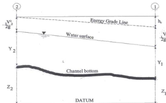
Fig. 2: Components in the energy equation. (Source: Chow et al. 1989).
