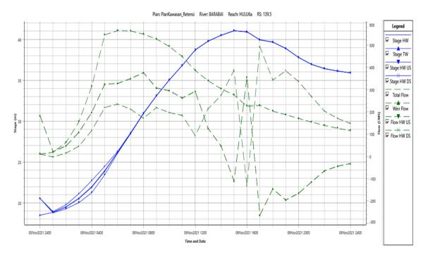
Fig. 7: Simulation of flow in regulation pool with 40% discharge. (Source : Calculation Result, 2021)
