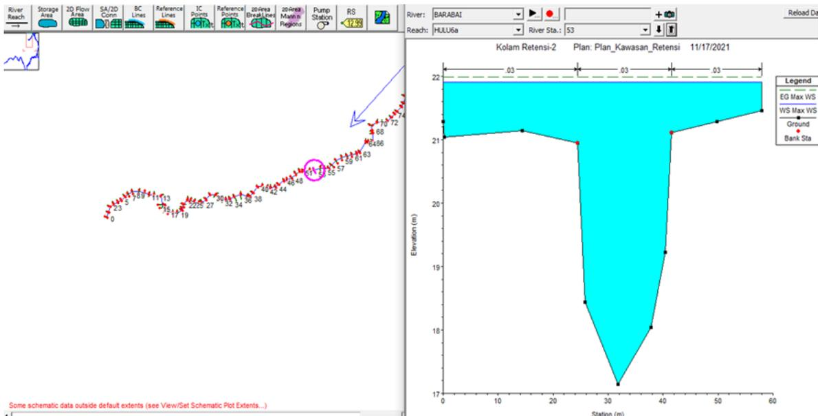
Fig. 11: Water level profile at STA 53 with 60% discharge. (Source: Calculation result, 2021).
