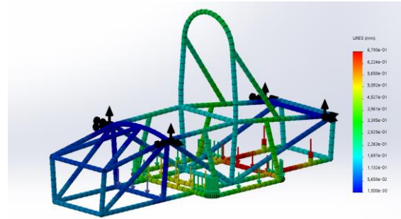
Gambar 14. Hasil Displacement Material Alluminium 6061-T6
