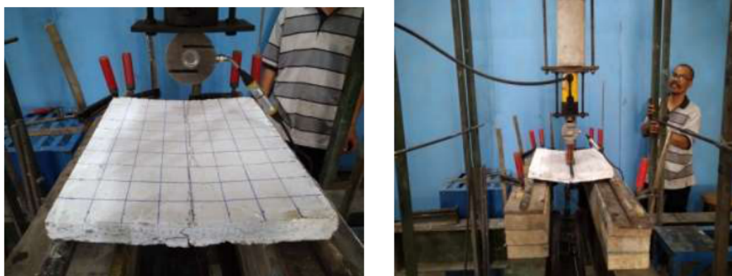
Figure 6 The testing process and cracks that occur during testing
