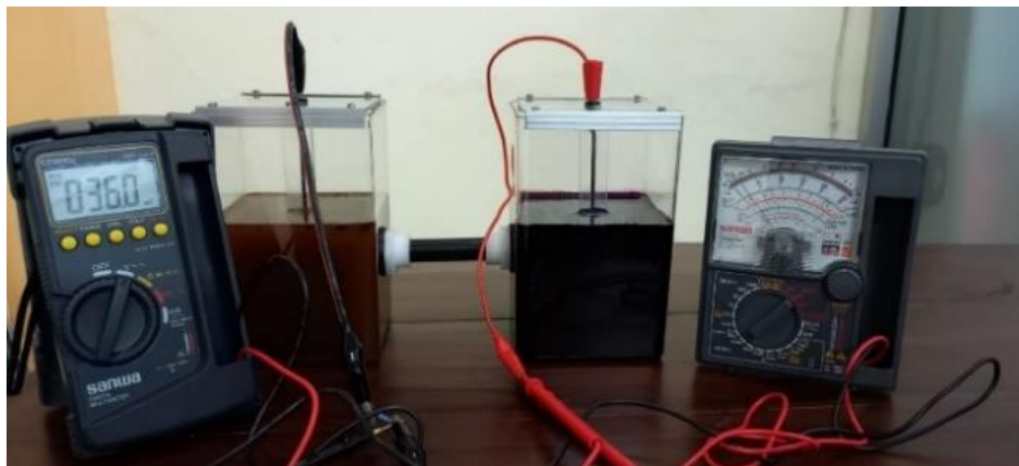
Figure 3 Voltage and Current Measurements in Cocoa Pod Waste MFC
