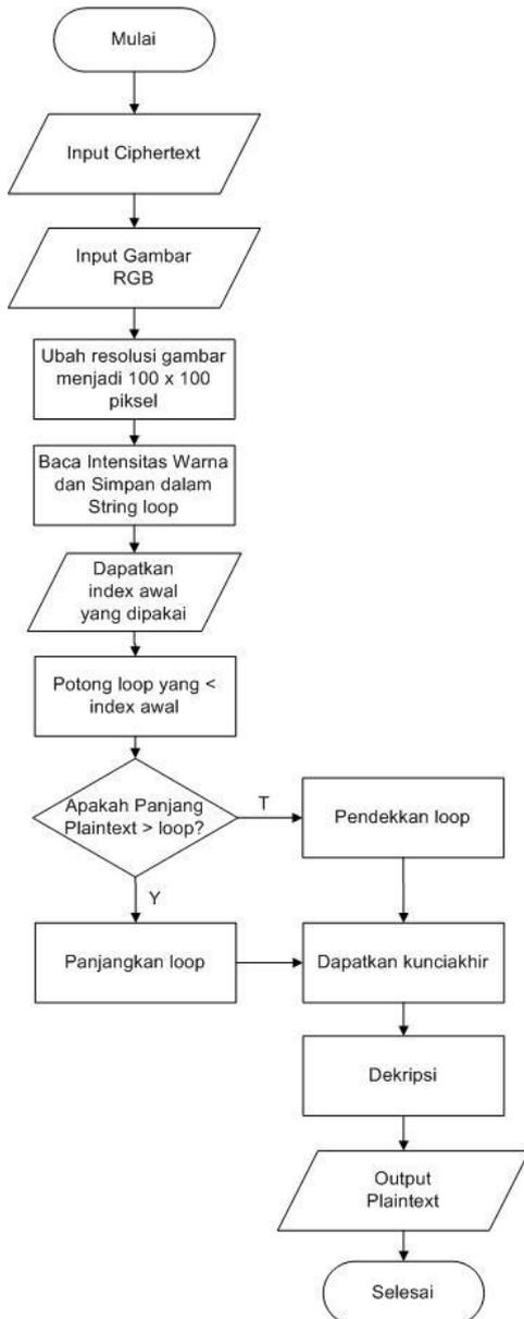
Gambar 3.3 Diagram Alur Proses Dekripsi
