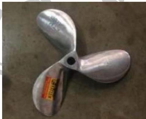
Gambar 1.1. Fixed Pitch Propellers berdaun 3 (Endrawan,2019)
