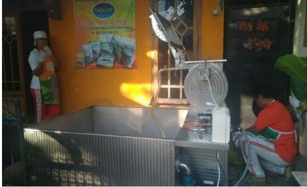
Figure 2. Adjusting the Components of a Vacuum Frying Machine
