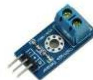
gambar 2.5 Sensor Tegangan
