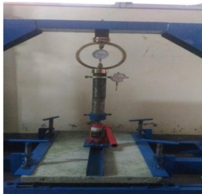
Fig 4. Diagram and Result of concrete water gate collapse test
