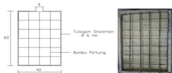
Fig 1. Selection of bamboo petung and how to mount reinforcement
