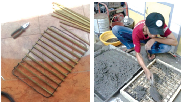
Figure 3: The process of making water gates from panels with reinforcement from bamboo
