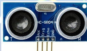
Gambar 2.4. Sensor Ultrasonik HC-SR04
