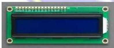
**Gambar 2.9** LCD (Liquid Cristal Display)
