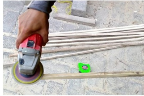
Fig. 3. Tidying a bamboo bar with a grinding machine.
