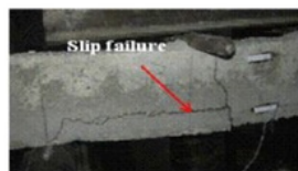
Fig. 29. Failure of bond-slip of the BRC beam [21].
