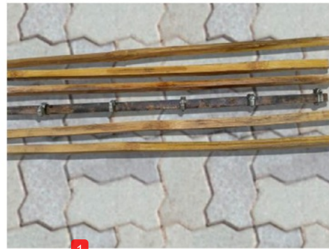
Fig. 4. Processing a waterproof coating, a sand coating, and a hose-clamp installation.
