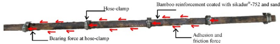
Fig. 1. Bamboo reinforcement with a hose-clamp.
