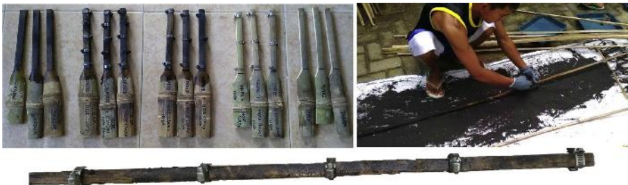
Fig. 11. Fine sand surfacing (volcanic dust from Raung Mountain, Jember, Indonesia).
