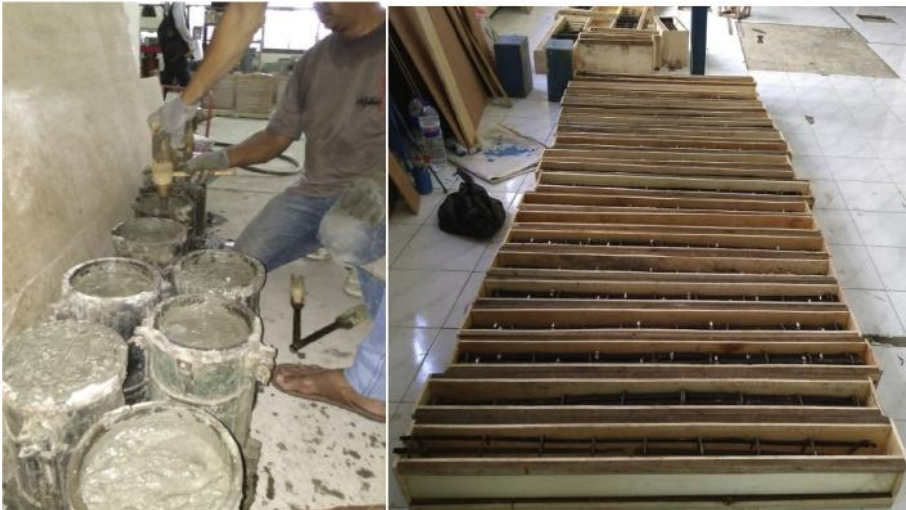
Fig. 12. Preparing pull-out test and flexural test specimens.
