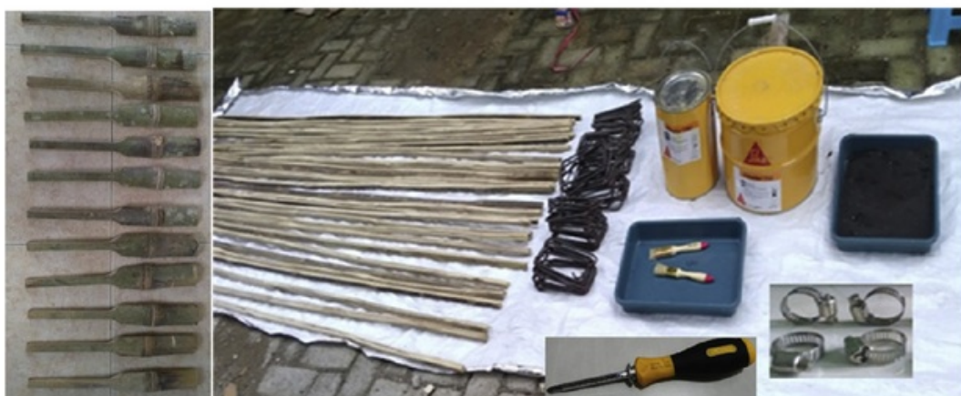
Fig. 8. Bamboo reinforcement of bamboo, Sikadur®-752, fine sand, hose-clamps, brushes, and steel stirrups.
