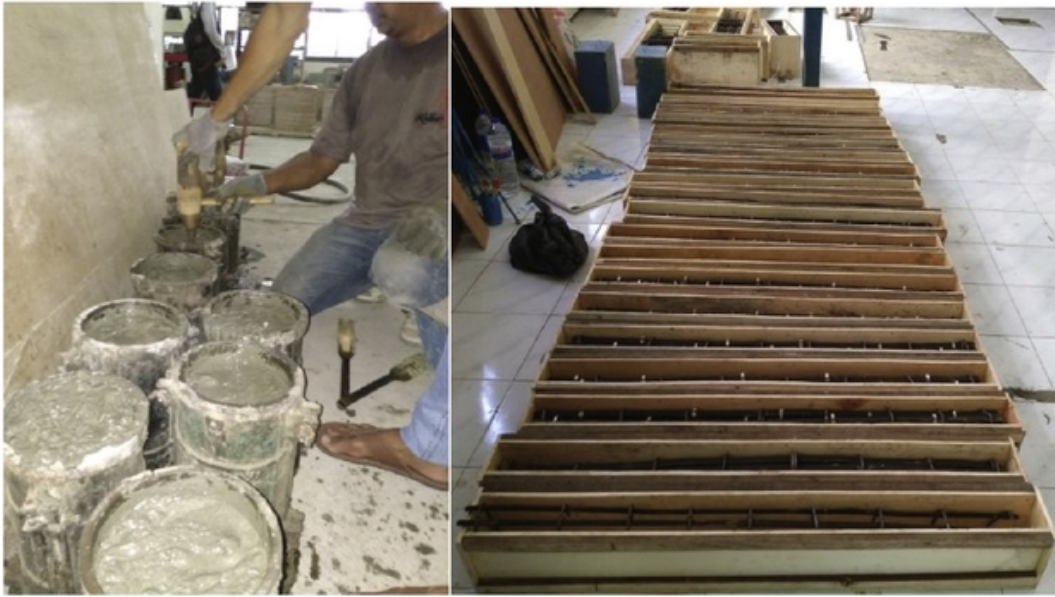
Fig. 12. Preparing pull-out test and flexural test specimens.
