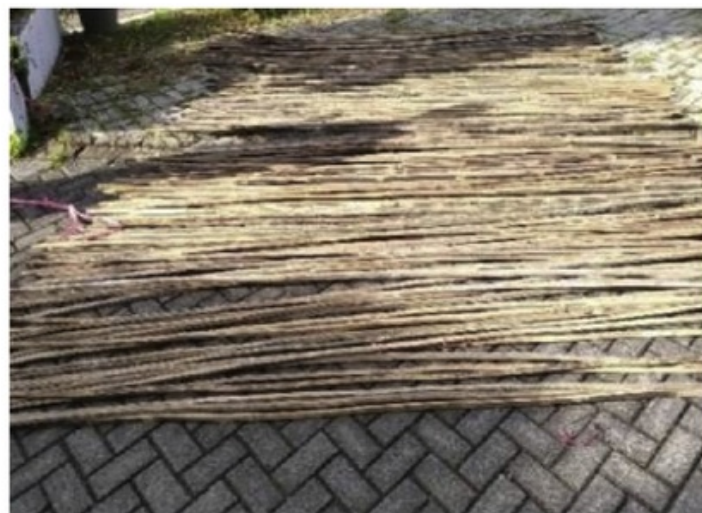
Fig. 5. Drying of bamboo in free air for \pm 1 month after soaking.
