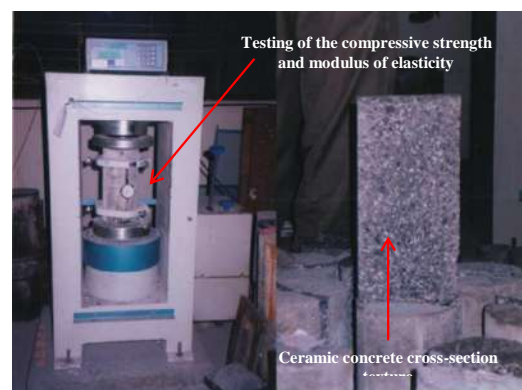
Fig. 2. Testing of the compressive strength and modulus of elasticity
