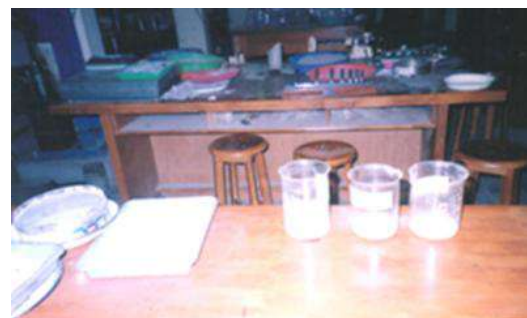
Fig. 3. Testing of the soundness or weathering on ceramic waste aggregates.
