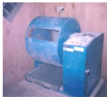
Fig. 5. Testing of the abrasion and impact on ceramic waste aggregates.
