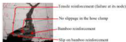
Figure 21 Failure on bamboo reinforcement BRC beam
