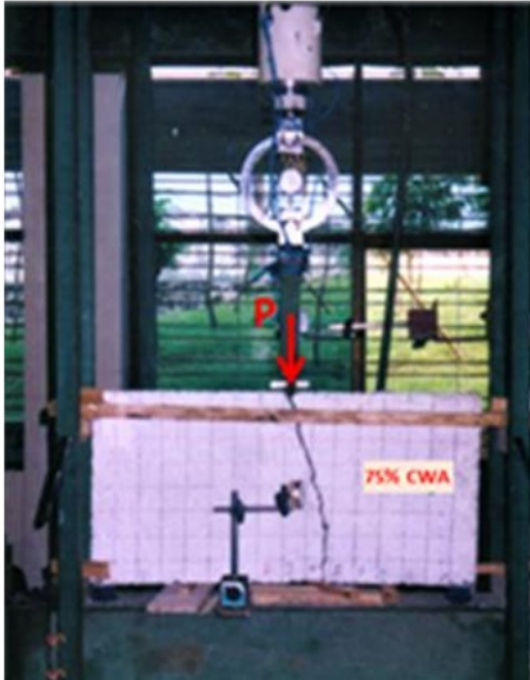
Fig. 8. The crack pattern of ceramic concrete panels (75% CWA)
