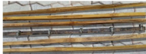
Fig. 3. Bamboo bars with waterproof and sand coating, and the hose clamp.
