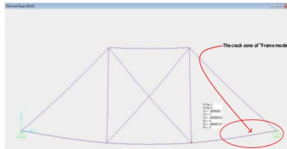
Fig. 10. The deformation of the rigid portal model or "Frame model"
