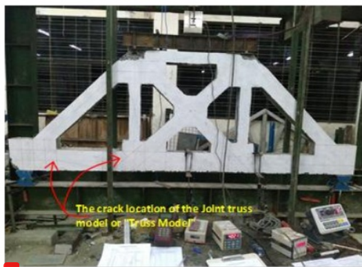
Fig. 7. The crack pattern of the joint truss model or "Truss Model"
