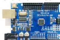
Gambar 2.1 Arduino UNO R3 ( Sumber : www.tweaking4all.com )
