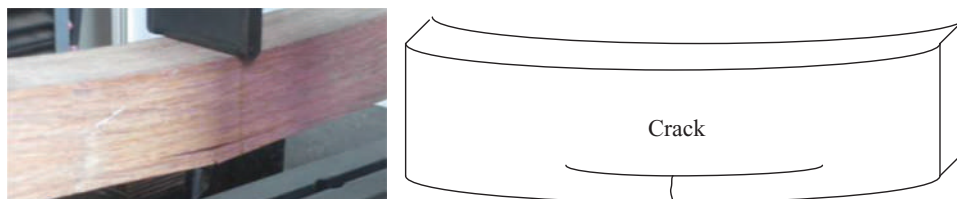
Figure 10: Typical failure mode for bending specimens
