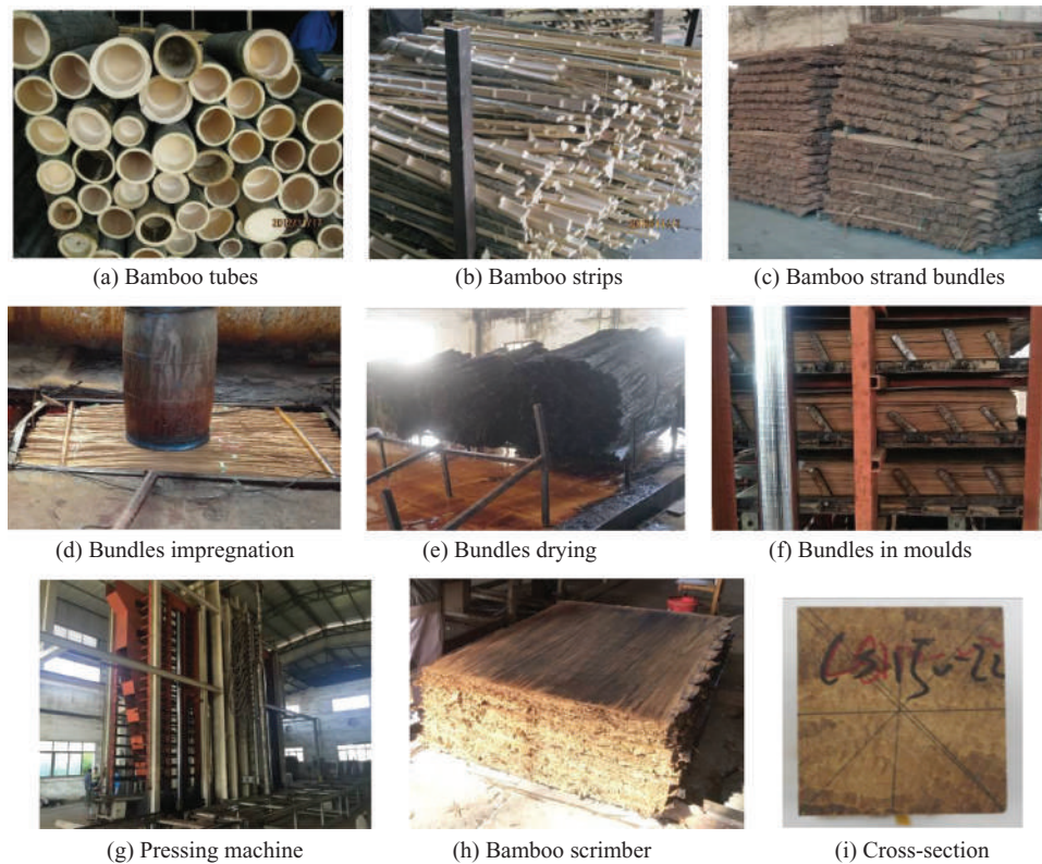
Figure 1: Main manufacturing process for bamboo scrimber
