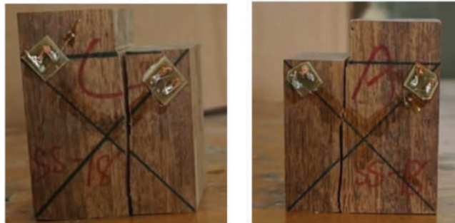
Figure 12: Typical failure mode for shear specimens
