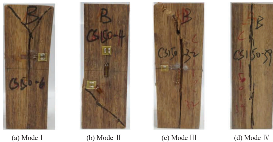
Figure 9: Typical failure modes for axial compression specimens
