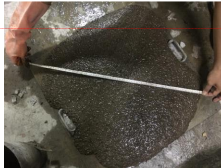
Gambar 3. Gambar Uji Slump Flow
