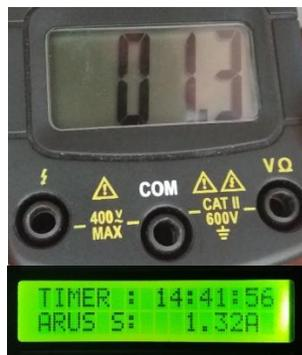
**Gambar 4.8** Kalibrasi Sensor Arus Non-Invasive Pada Phase S
