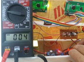
**Gambar 4.3** Pengujian Rangkaian Regulator Step Down
