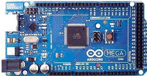
**Gambar 2.7** Arduino Mega 2560
