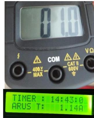
**Gambar 4.9** Kalibrasi Sensor Arus Non-Invasive Pada Phase T.
