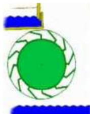
Gambar 2.2. Kincir air Overshot (Sumber : Haimeri, L.A., 1960)
