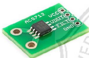
Gambar 2.5 Sensor arus ACS712
