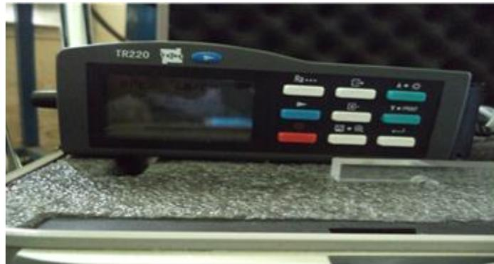
Gambar 1. alat ukur *surface roughness tester TR220*
