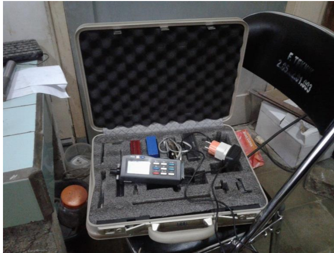
Gambar 1. alat ukur surface roughness tester TR220
