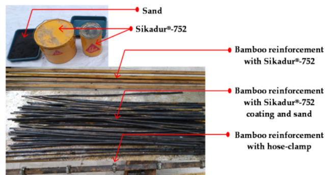
Figure 1. The materials and treatments of bamboo reinforcement.
