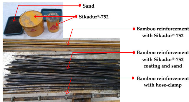
Figure 1. The materials and treatments of bamboo reinforcement.
