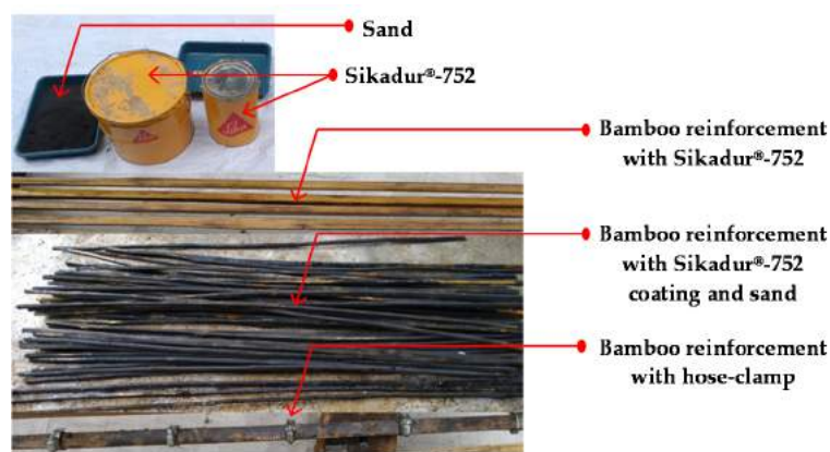
Figure 1. The materials and treatments of bamboo reinforcement.
