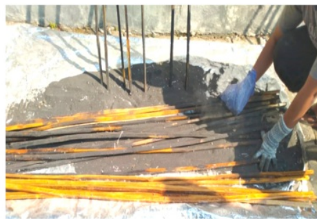
Figure 7. Sand sprinkling on bamboo reinforcement.
