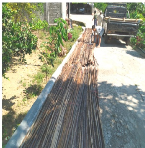
Figure 4. Drying bamboo in free air.
