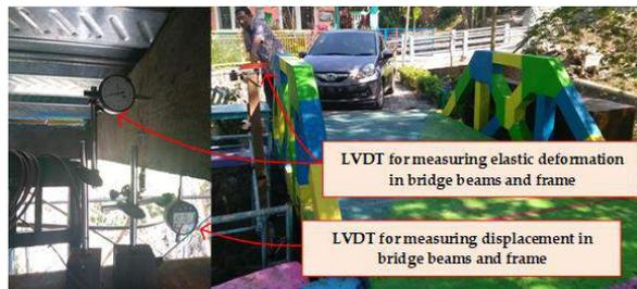
Figure 30. The measuring the elastic displacement and deformation.
