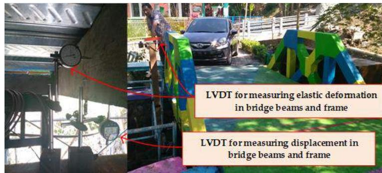
Figure 30. The measuring elastic displacement and deformation
