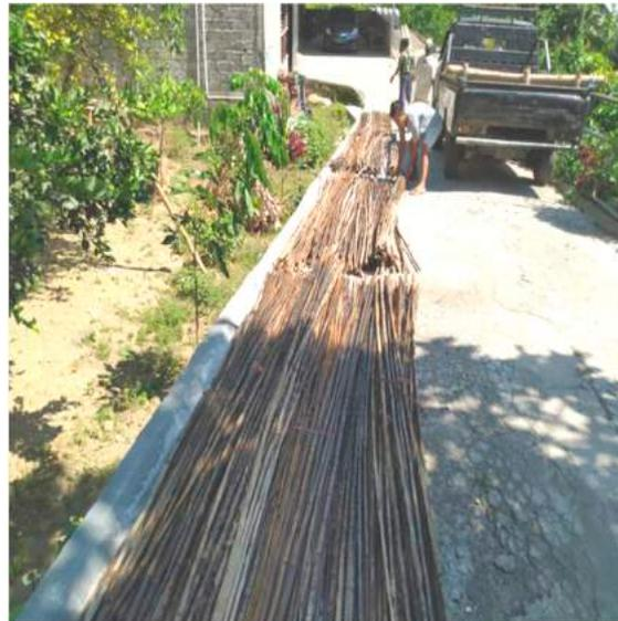
**Figure 4.** Drying bamboo in free air.
