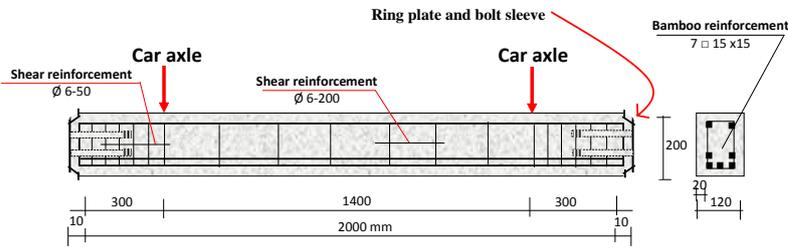
Figure 13. Details of the precast bridge beam reinforcement [12].
