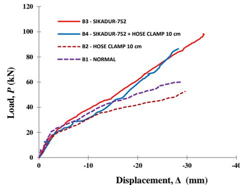
Figure 1. The relationship of Load vs. deflection of BRC beam [12]
