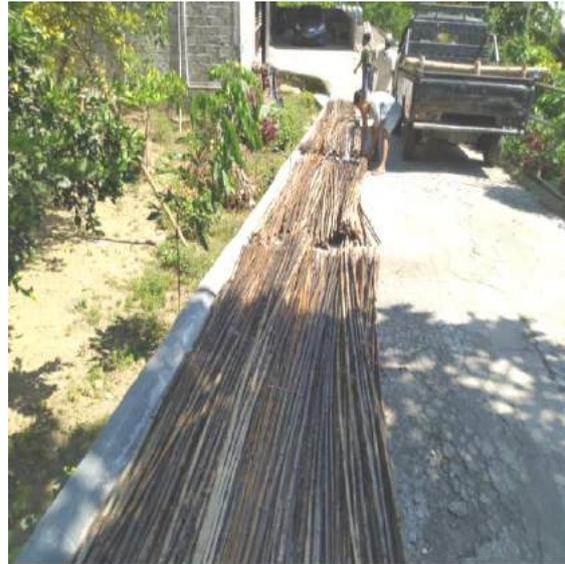
**Figure 4.** Drying bamboo in free air
