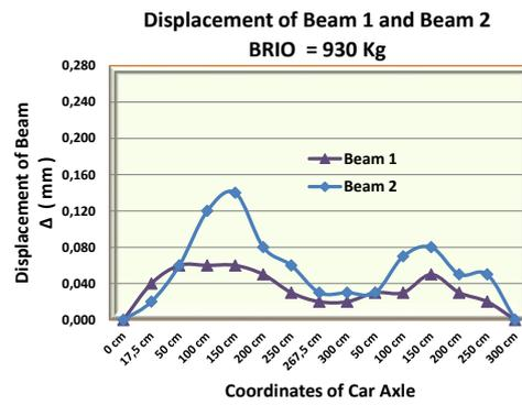
Figure 25. Displacement of the beam with loads of BRIO car of no passengers
