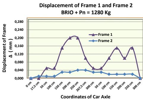
Figure 22. Displacement of the frame with loads of BRIO car of full passengers
