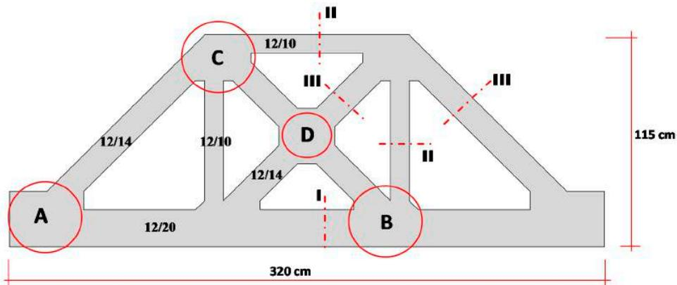
Figure 13. Details of the precast bridge frame [38].
