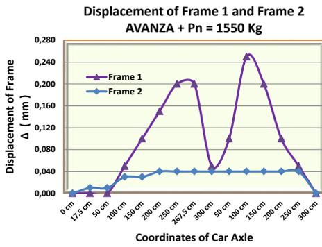
Figure 20. Displacement of the frame with loads of AVANZA car of full passengers
