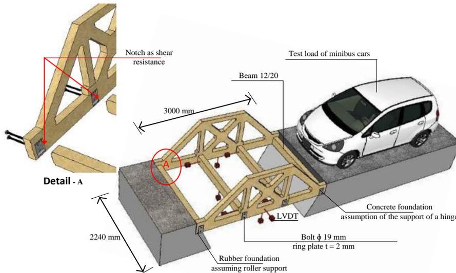
Figure 18. Arrangement of testing for bamboo reinforced concrete frame precast bridges
