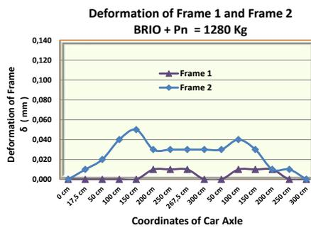
Figure 28. Deformation of the frame with loads of the BrioRIO car of full of passengers.
