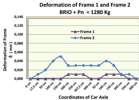
Figure 28. Deformation of the frame with loads of the Brio car full of passengers.
