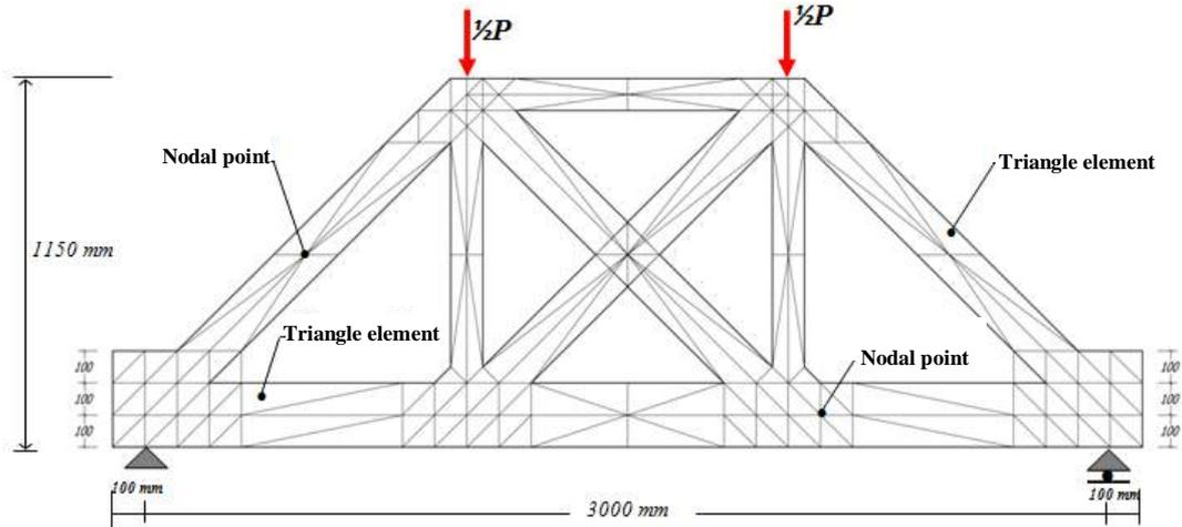
Figure 31. Discretization of Bamboo Reinforced Concrete Bridge Frames
