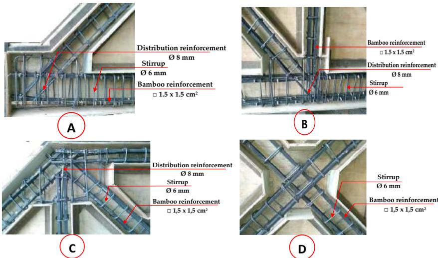
Figure 15. Details of the knot reinforcement for the bridge frames [23].
