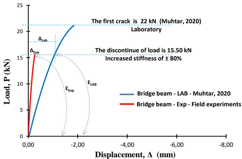
Figure 36. The relationship of load vs. displacement of bridge beam from laboratory test results and field experiment results
