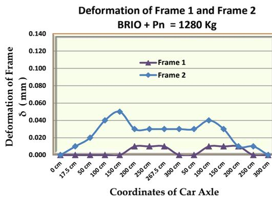
Figure 28. Deformation of the frame with loads of the Brilio car full of passengers.
