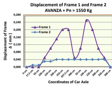
Figure 20. Displacement of the frame with loads of the AvanzaVANZA car of full of passengers.
