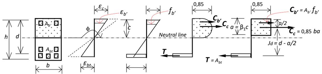
Figure 9. Stress-strain distribution diagram in a BRC beam
