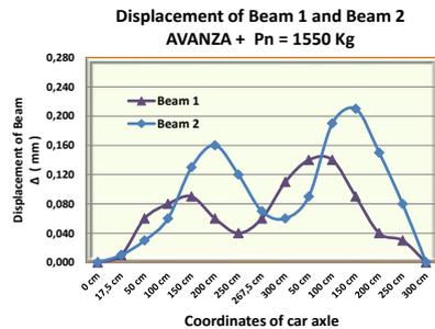
**Figure 21.** Displacement of the beam with loads of the Avanza car full of passengers.
