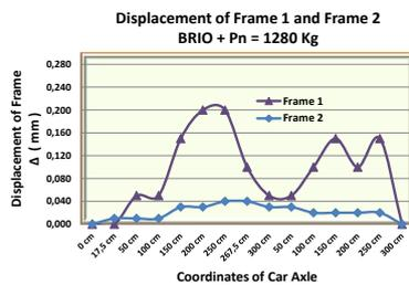
Figure 22. Displacement of the frame with loads of the BRIO car of full of passengers.
