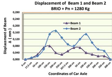
Figure 23. Displacement of the beam with loads of the BRIO car of full of passengers.
