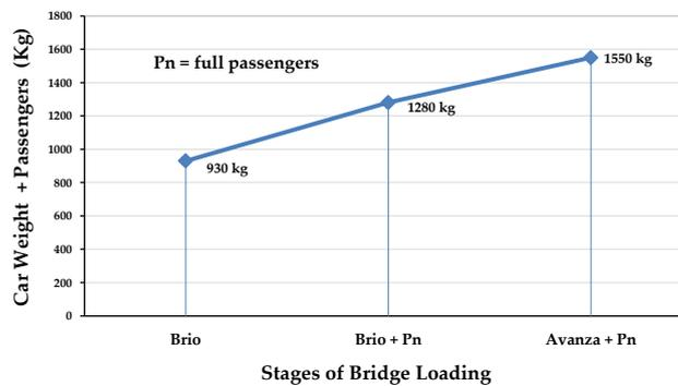
Figure 16. Loading stage of precast bridges of bamboo reinforced concrete frame
