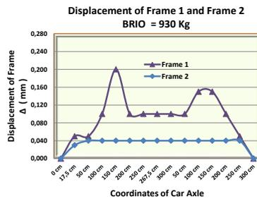
Figure 24. Displacement of the frame with loads of the BRIO car of with no passengers.
