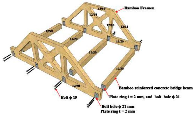
Figure 11. Model of the precast bridge made from bamboo reinforced concrete.
