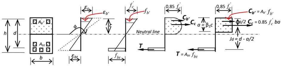
Figure 11. Stress–strain distribution diagram in a BRC beam [1,22].
