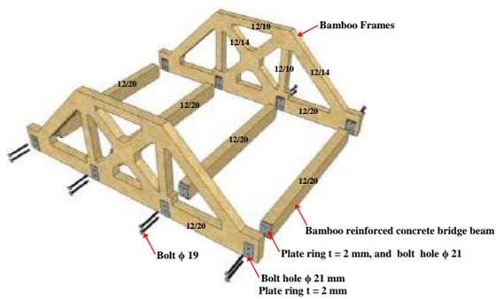
Figure 12. Model of the precast bridge made from bamboo-reinforced concrete.
