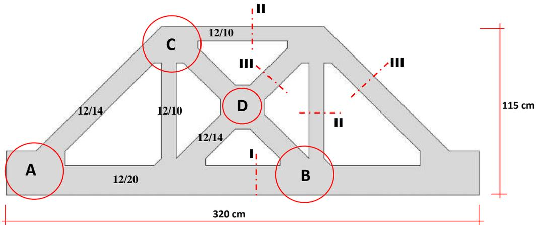
Figure 14. Details of precast bridge frame [23]
