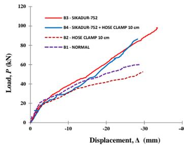
Figure 1. The relationship of Load vs. deflection of the bamboo-reinforced concrete (BRC) beam [12].
