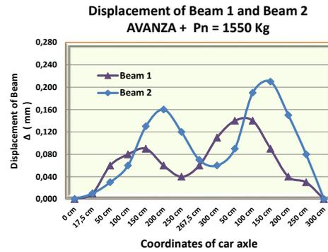
Figure 21. Displacement of the beam with loads of AVANZA car of full passengers
