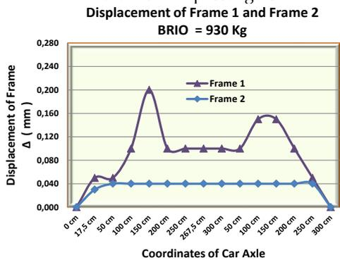
Figure 24. Displacement of the frame with loads of BRIO car of no passengers
