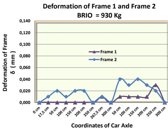
Figure 27. Deformation of the frame with loads of BRIO car of no passengers
