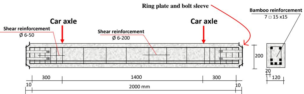
Figure 13. Details of Precast bridge beam reinforcement [12]
