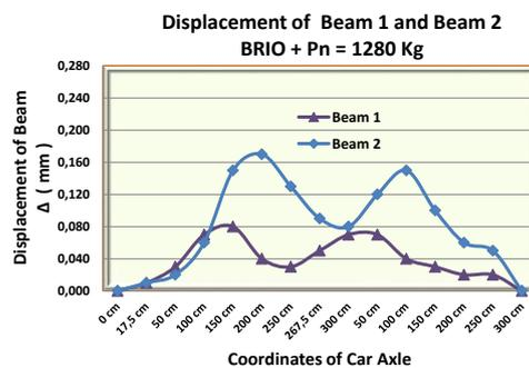
Figure 23. Displacement of the beam with loads of BRIO car of full passengers
