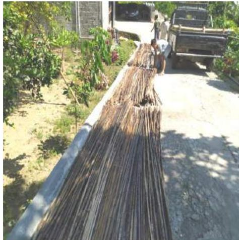
**Figure 4.** Drying bamboo in free air.
