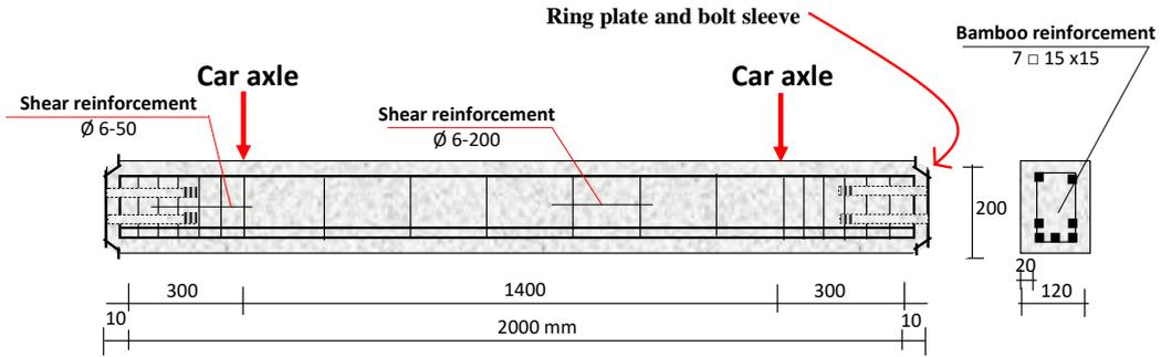
Figure 13. Details of Precast bridge beam reinforcement [12]
