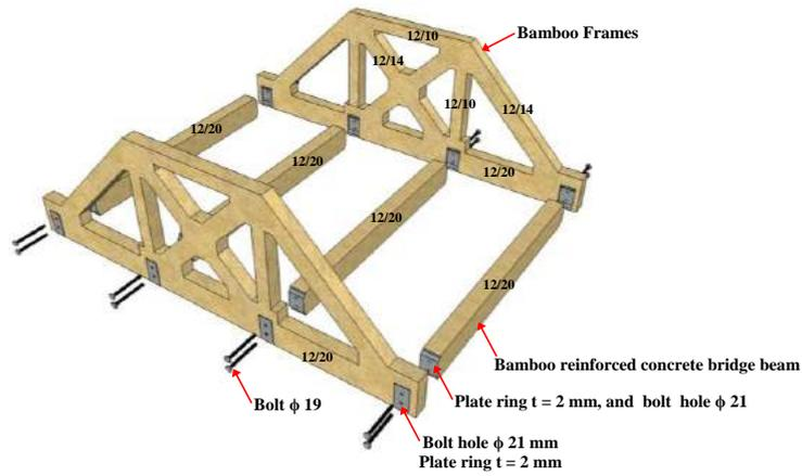
Figure 12. Model of the precast bridge from bamboo reinforced concrete
