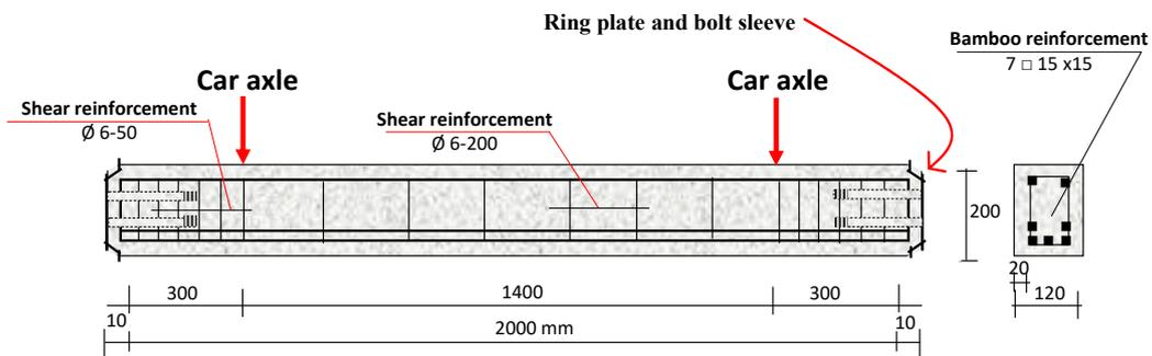
Figure 12. Details of the precast bridge beam reinforcement [22].
