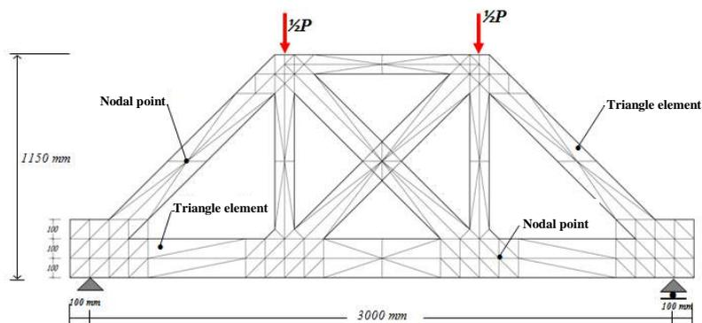
Figure 31. Discretization of the bamboo-reinforced concrete bridge frames.
