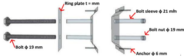
Figure 10. Details of ring plate and bolt sleeve
