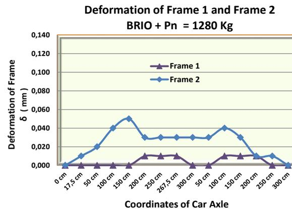
Figure 28. Deformation of the frame with loads of BRIO car of full passengers
