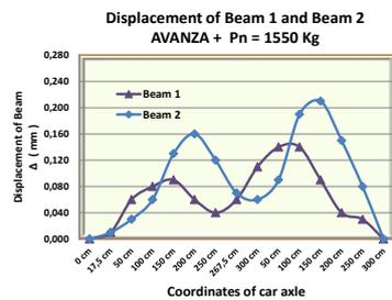
Figure 21. Displacement of the beam with loads of the AvanzaVANZA car of full of passengers.
