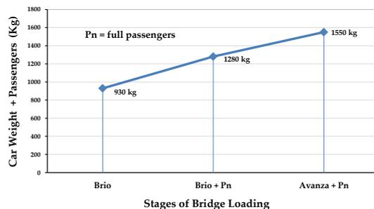
Figure 16. Loading stage of the precast bridges with a bamboo reinforced concrete frame.
