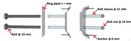
Figure 10. Details of ~~the~~ ring plate and bolt sleeve.
