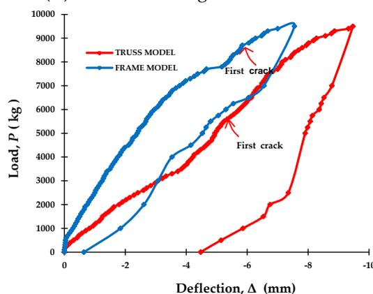
Figure 2. The relationship pattern of load vs. deflection of the bridge frame [23]
