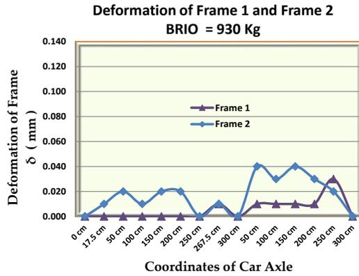
Figure 27. Deformation of the frame with loads of the Brilio car with no passengers.
