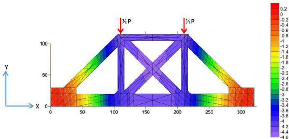
Figure 32. The displacement of Y-direction of the bridge frame
