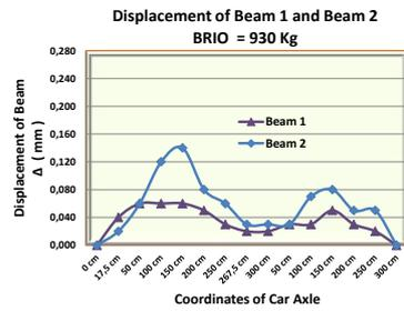
Figure 25. Displacement of the beam with loads of the BRIO car of with no passengers.
