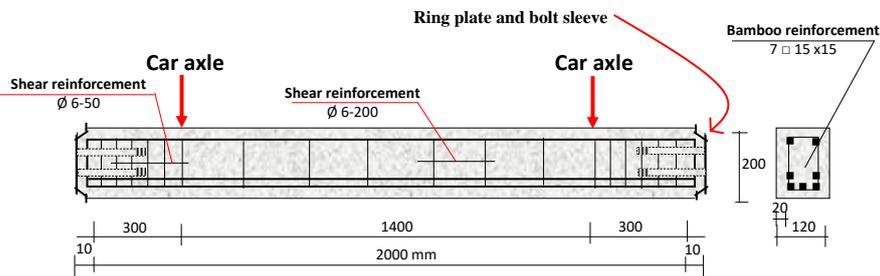
Figure 13. Details of the precast bridge beam reinforcement [22].
