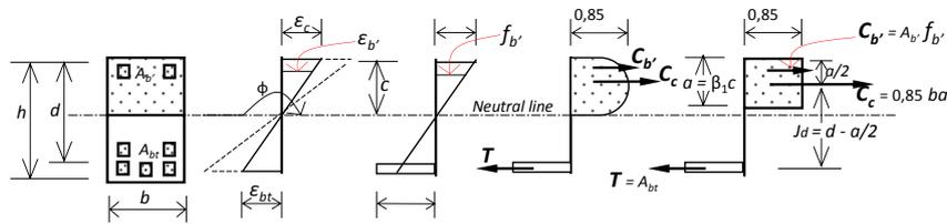
Figure 9. Stress-strain distribution diagram in a BRC beam [1,12].
