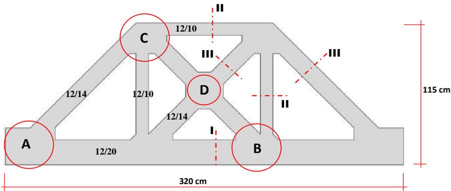
Figure 14. Details of the precast bridge frame [23].
