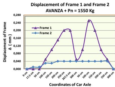
**Figure 20.** Displacement of the frame with loads of the Avanza car full of passengers.
