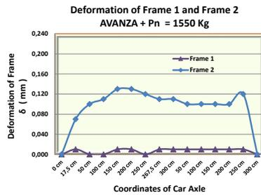
Figure 29. Deformation of the frame with loads of the AvanzaVANZA car of full of passengers.
