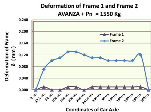
Figure 29. Deformation of the frame with loads of AVANZA car of full passengers
