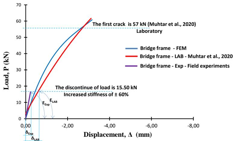
Figure 35. The relationship of load vs. displacement of bridge frame from laboratory test results, FEM results, and field experiment results
