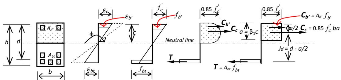
Figure 15. Stress–strain distribution diagram in a BRC beam [1,22].
