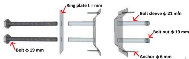
Figure 10. Details of ring plate and bolt sleeve
