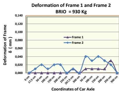
Figure 27. Deformation of the frame with loads of the BrioRIO car with no passengers.
