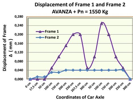
Figure 20. Displacement of the frame with loads of AVANZA car of full passengers
