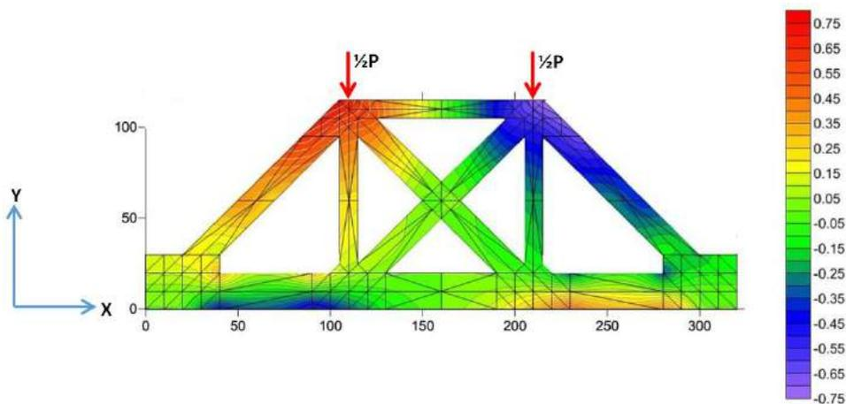
Figure 33. The displacement of X-direction of the bridge frame
