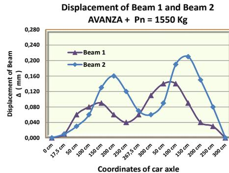
Figure 21. Displacement of the beam with loads of AVANZA car of full passengers
