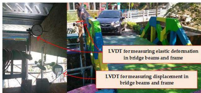
Figure 30. Measuring the elastic displacement and deformation.
