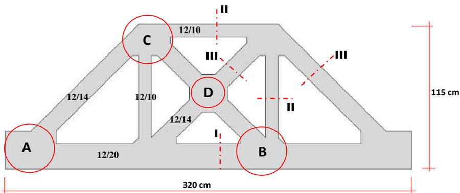
Figure 14. Details of the precast bridge frame [38].
