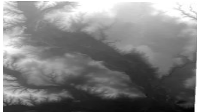
Fig. 8. Watershed Transformation Results with 30 meter DEM SRTM Data (Condition 2)
