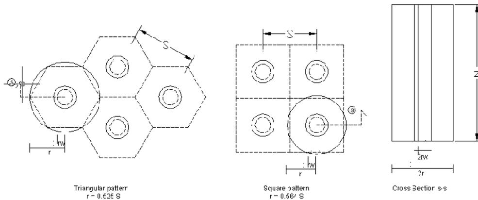
Gambar 2.3. General Lay out of vertical sand drain
